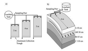
Fig. 1 Schematic diagram of (a) vegetative filter strips of 2 m width  $\times$  3, 4, and 5 m length. Leachate was applied uniformly across each VFS and runoff was collected in aluminum trays. The same leachate application system was used for subsurface experiments (b). Aluminum trays (width = 1 m) were placed at different soil horizon interfaces to capture discharge. The horizon name and depth are listed.
